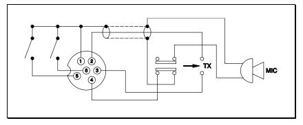
Transceiver Microphone Schematic Diagram
